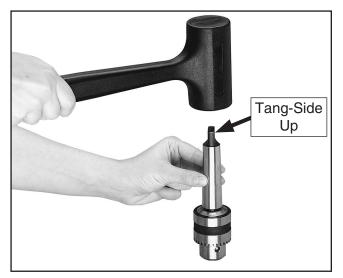
Figure 16. Seating arbor into chuck.
